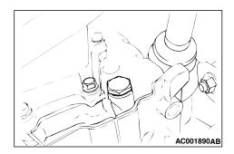
3. Remove the drain plug from the bottom of the transaxle case to drain the A/T fluid.
